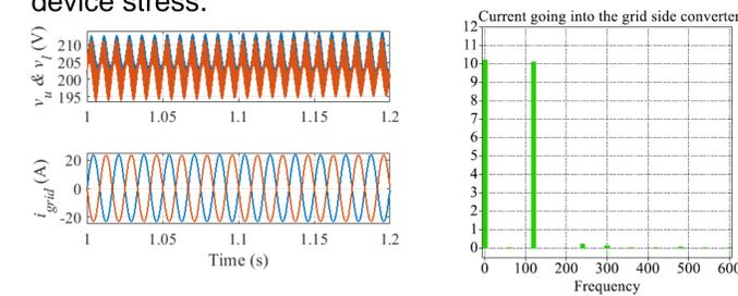
Fig. 5 – Voltage across upper and lower capacitor and current injected into grid.
