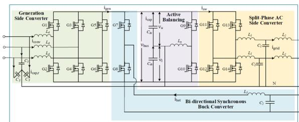
Fig. 2 – Proposed multi-port converter topology.
