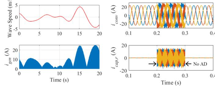
Fig. 3 – Wave speed profile and oscillatory current injection into the DC bus.
