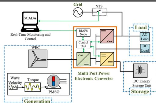
Fig. 1 – Marine microgrid with multi-port power electronic converter.
